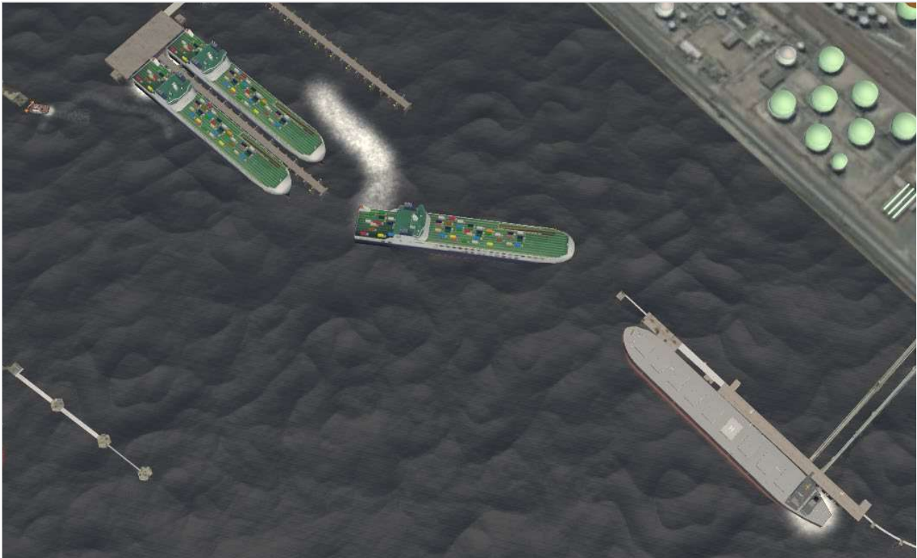
Figure 4.15: Run 19 showing limited manoeuvring space between new infrastructure and end of Immingham East Jetty
